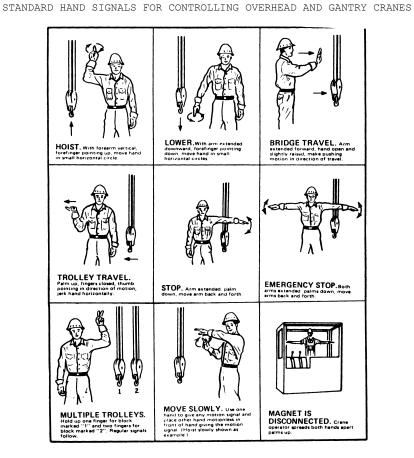
(3) The following hand signals must be used for derricks and a copy must be posted in the cab at the operator's station.
